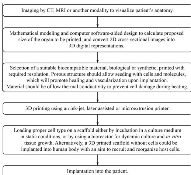
Fig. 1. The procedure of 3D printing human organs.
