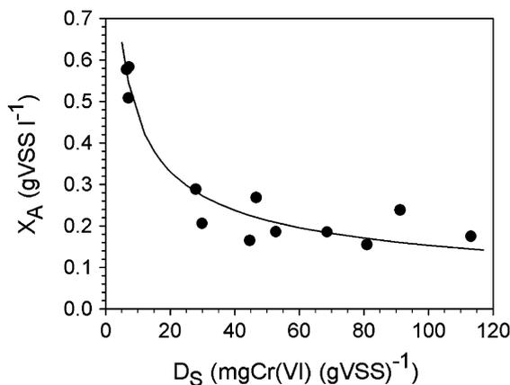
Fig. 4. Active biomass concentration of *S. natans* as a function of the ratio between influent Cr(VI) concentration and biomass concentration in steady state condition of the bioreactor operated under continuous regime limited in CES ( $D = 0.065\text{--}0.24 \text{ h}^{-1}$ ). (—) Predictions by Eq. (10).
