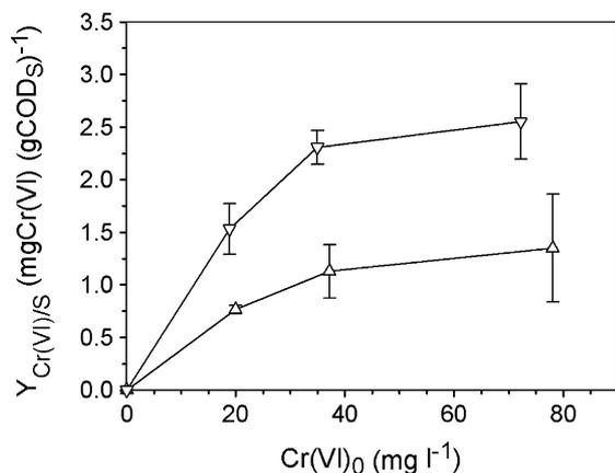
**Fig. 7.** Cr(VI) reduction yield ( $Y_{\text{Cr(VI)/S}}$ ) as a function of the initial Cr(VI) concentration for the assayed ranges of biomass concentration in batch tests ( $\text{mgVSS l}^{-1}$ ): ( $\Delta$ ) 170–190; ( $\nabla$ ) 400–500. The standard deviations are indicated by error bars.
