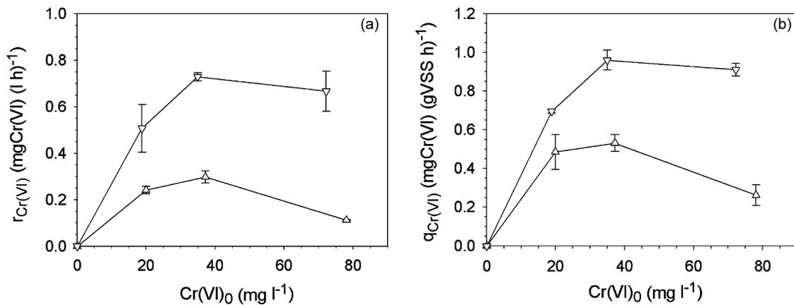
**Fig. 6.** Cr(VI) reduction for *S. natans* growing in batch bioreactor with different initial Cr(VI) concentration and ranges of biomass concentration ( $\text{mgVSS l}^{-1}$ ): ( $\Delta$ ) 170–190; ( $\nabla$ ) 400–500. (a) Cr(VI) reduction rate ( $r_{\text{Cr(VI)}}$ ); (b) specific Cr(VI) reduction rate ( $q_{\text{Cr(VI)}}$ ). The standard deviations are indicated by error bars.
