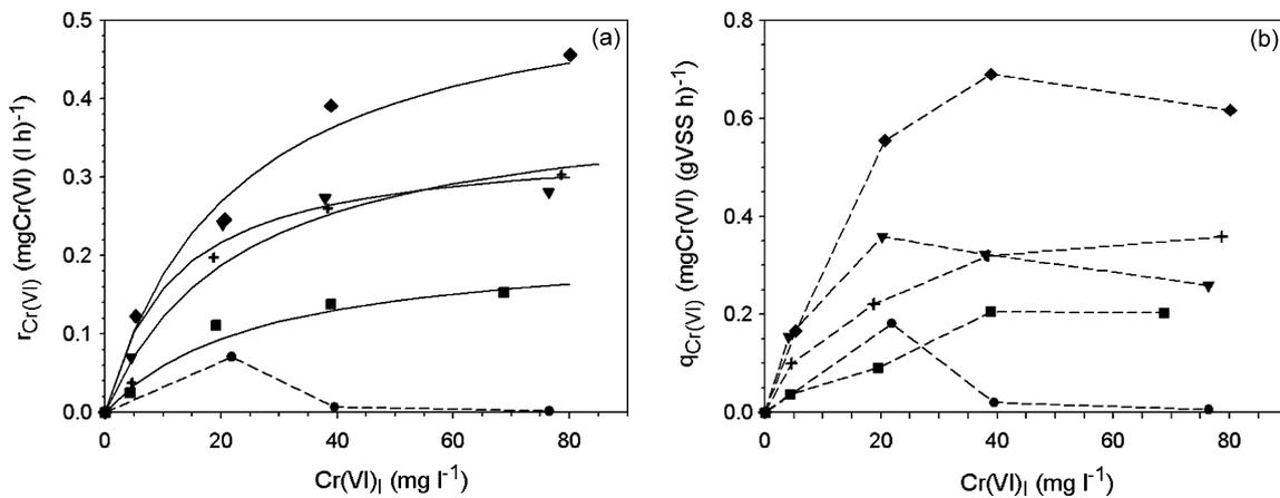
**Fig. 1.** Cr(VI) reduction for *S. natans* growing in continuous bioreactor at different dilution rates ( $D$ , h<sup>-1</sup>) and influent Cr(VI) concentration ( $Cr(VI)_i$ ): (a) Cr(VI) reduction rate ( $r_{Cr(VI)}$ ); (b) specific Cr(VI) reduction rate ( $q_{Cr(VI)}$ ). Continuous culture limited in CES:  $D$  = (●) 0.02, (■) 0.065, (▼) 0.12, (◆) 0.24; continuous culture limited in NS: (+) 0.11. (—) Predictions by Eq. (5).
