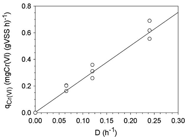
**Fig. 2.** Specific Cr(VI) reduction rate ( $q_{Cr(VI)}$ ) as a function of the dilution rate ( $D$ , h<sup>-1</sup>) for influent Cr(VI) concentration of the bioreactor ranging from 19.2 and 80.1 mg l<sup>-1</sup>.
