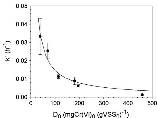
**Fig. 9.** Apparent chromium(VI) reduction coefficient ( $k'$ ,  $\text{h}^{-1}$ ) as a function of the ratio between initial Cr(VI) concentration and initial biomass concentration ( $D_0$ ,  $\text{mgCr(VI)}_0$  ( $\text{gVSS}_0$ ) $^{-1}$ ) for batch culture of *S. natans*. (●) Experimental data. (—) Predictions by Eq. (20).
