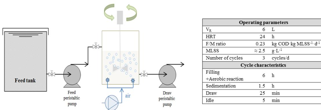
**Figure 1. SBRs characteristics and configuration.**
