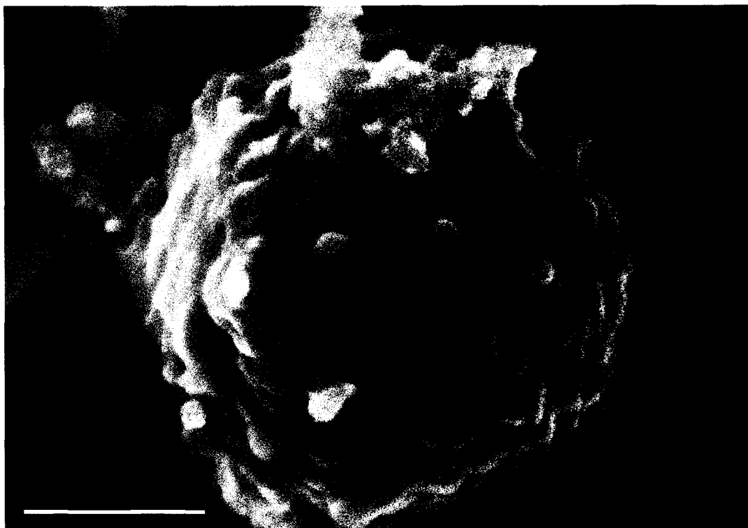
Figure A-2: An 11% w/w skim milk powder solution prepared on a carbon substrate imaged with the Hitachi S-4800. Bar = 100nm
