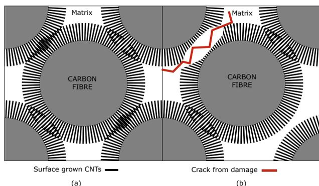
Figure 26: A schematic of pristine carbon fibres in matrix with surface grown carbon nanotubes (a), diagram of damaged surface nanotubes due to delamination or crack between the carbon fibre (b).
