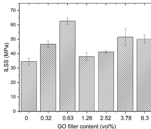
Figure 6: Graph of interlaminar shear strength of CFRP samples with increasing graphite oxide contents. Used with permission [24].
