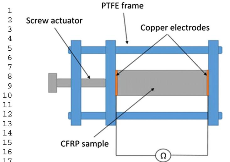
Figure 5: Diagram of the test fixture used for the electrical conductivity measurements used with permission. Used with permission [24].
