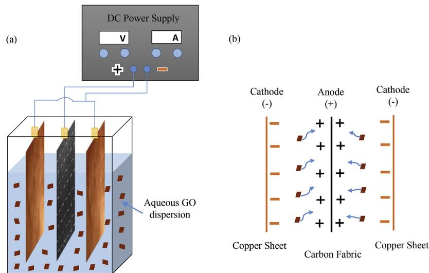
Figure 9: Schematic diagram of the electropheretic deposition technique used to coat carbon fibre plies (a) setup, (b) mechanism illustrating the deposition of graphene oxide. Used with permission [48].
