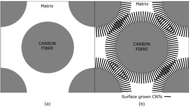
Figure 21: A schematic showing the cross sections of unmodified (a) and modified (b) carbon fibres.
