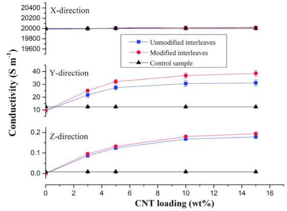
Figure 13: Results of conductivity measurements done by Li et al. [9] for the control (black) untreated (unmodified, blue), and plasma-treated (modified, red), for along fibre (X-direction), transverse (Y-direction) and through-thickness (Z-direction). Published by the royal society of chemistry [9].
