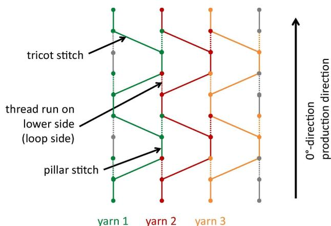
Figure 16: Knitting pattern of the silver coated polyamide, the tricot stitch refers to the stitch between the fibres and the pillar stitch is a winding or stitching around a single fibre. Used with permission [8].
