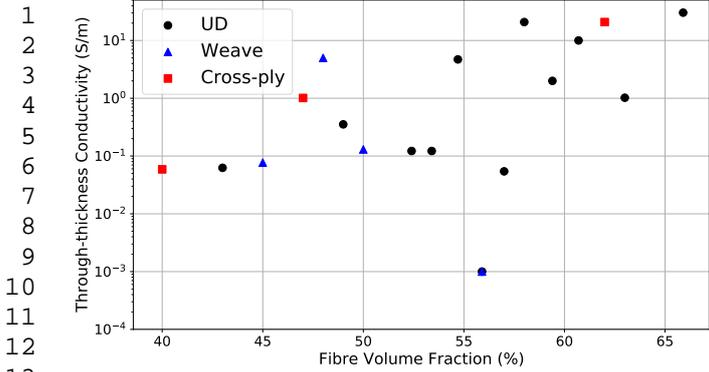
Figure 17: Graph of the variation of the through-thickness conductivity with the fibre volume fraction of the unmodified CFRPs. Data was taken from multiple papers that discuss through-thickness conductivity in Epoxy based CFRPs [4, 8, 9, 21, 22, 24–26, 36, 63, 72, 73, 76, 77, 82, 83]
