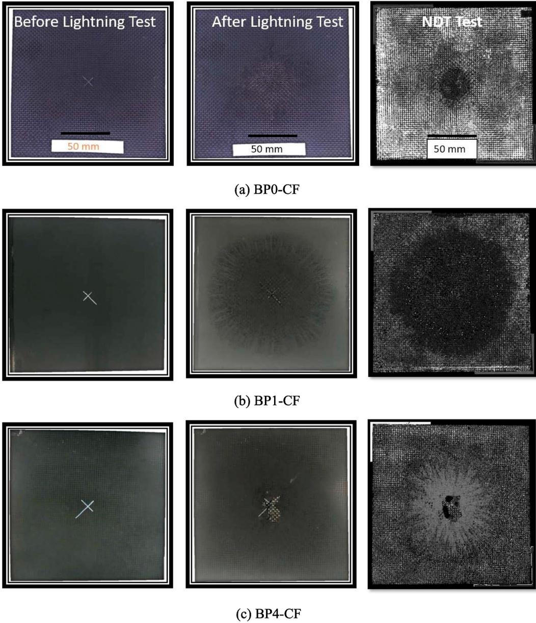
Figure 15: CFRP specimens before & after lightning strike and NDT images taken using a Scanning Acoustic Topograph connected to a 5MHz transducer (a) BP0-CF (b) BP10-CF and (c) BP4-CF. Used with permission [4].
