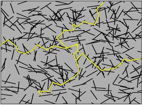
Figure 19: A schematic of percolation through a high aspect ratio particle network.
