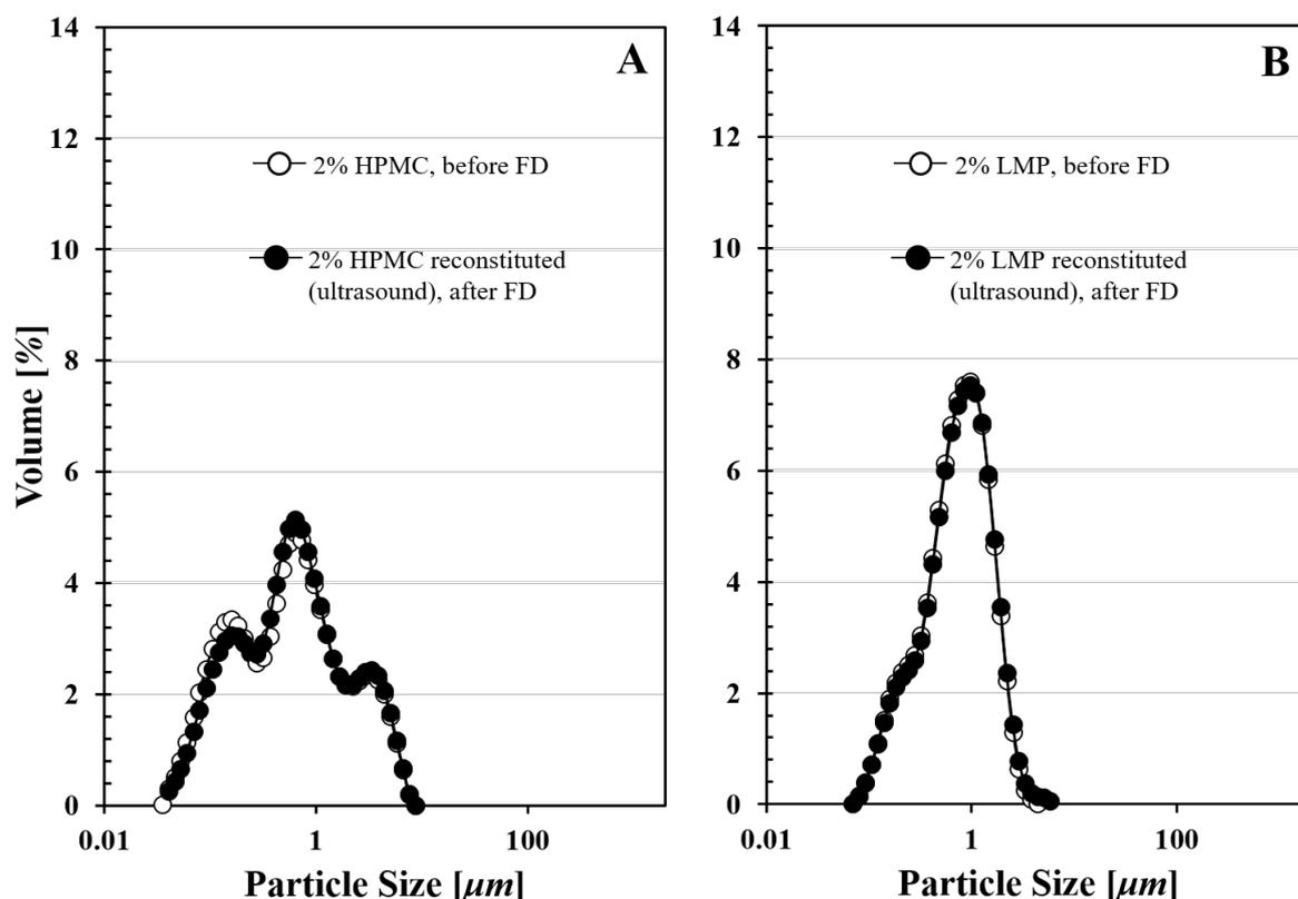
**Fig. 3.** Solid cetyl palmitate particles fabricated in the presence of 2 %wt HPMC (A) and 2 %wt LMP (B) before and after freeze-drying.
