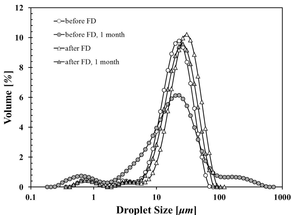
**Fig. 11.** 20 wt% o/w emulsions formed with dried and rehydrated 2.5 wt% wax particles and 0.8 wt% NaCas stored for different times at refrigeration temperatures. The same emulsions produced with non-freeze-dried particles are also included for comparison.
