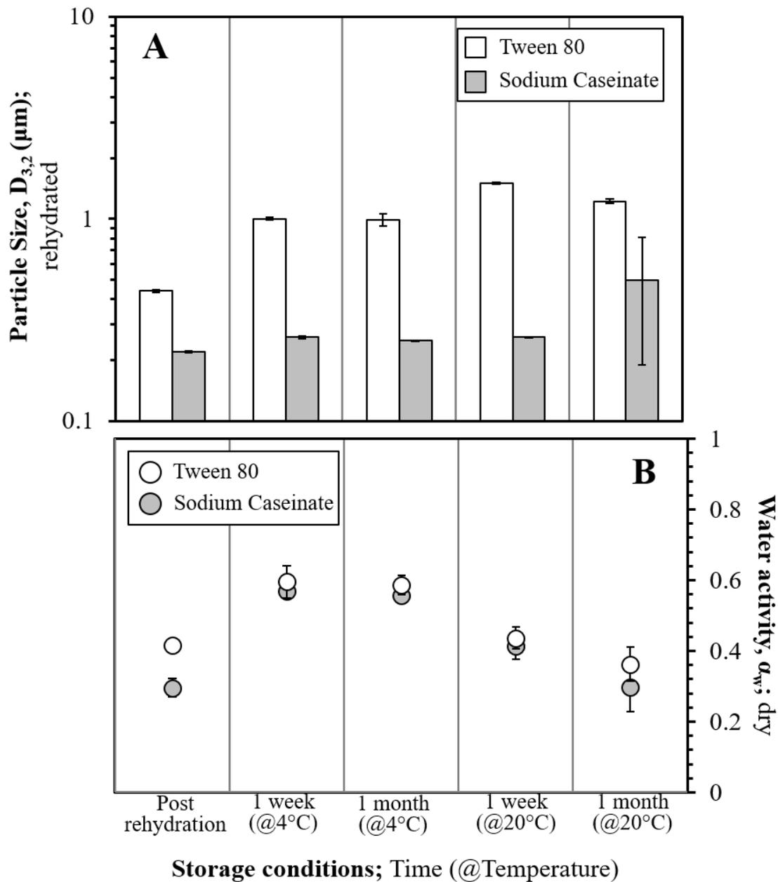
**Fig. 7.** Size properties (A) of redispersed cetyl palmitate particles formed with 0.8% Tween 80 or sodium caseinate under different storage times and conditions. Water activity of these systems measured in dry state (B).
