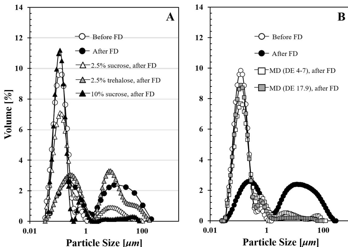
**Fig. 4.** Particle size distributions of 2.5 %wt solid cetyl palmitate particles produced with 0.8 % wt Tween 80 after reconstitution of the lyophilised samples in the presence of sucrose and trehalose as cryoprotectants at different concentrations (A), as well as different DE maltodextrins (MD) at 2.5 %wt concentration (of the final dispersion) (B).
