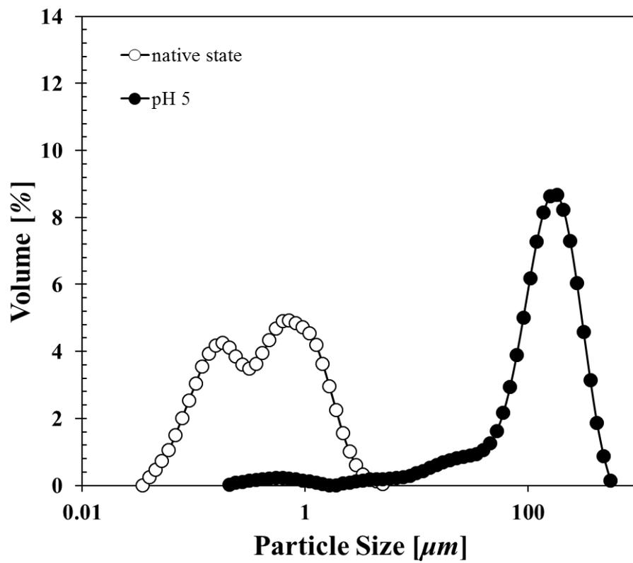
Fig. S1. Effect of protein's pH on lipid particle's redispersion behaviour. Size distributions refer to cetyl palmitate particles formed with 0.8% NaCas.
