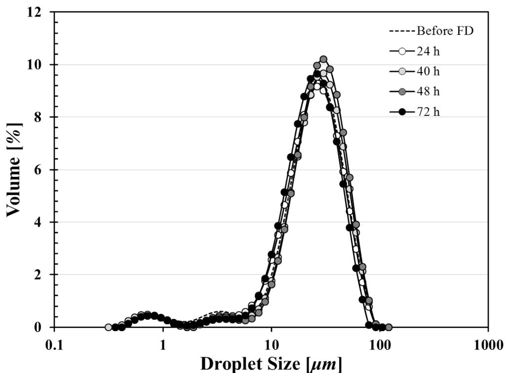
**Fig. 10.** Droplet size distribution curves for 20% sunflower oil emulsions formed with dried and reconstituted 2.5% wax particles and 0.8% NaCas for different drying times. The same emulsions produced with non-freeze-dried particles are also included for comparison.
