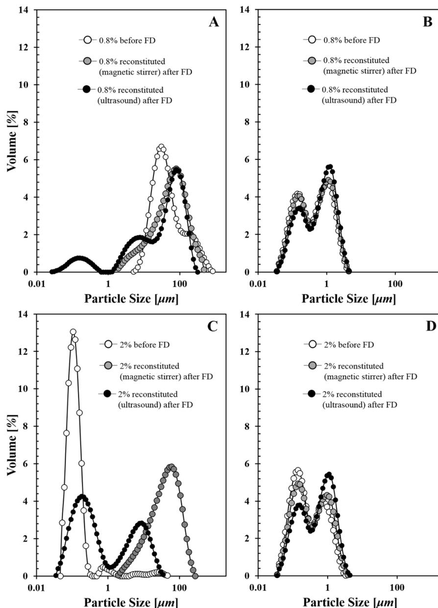
**Fig. 2.** Particle size distributions of solid tristearin (triglyceride) particles formed with 0.8 and 2%wt Tween 80 (A, C) and sodium caseinate (B, D) before and after freeze-drying (FD) and for two different reconstitution methods.
