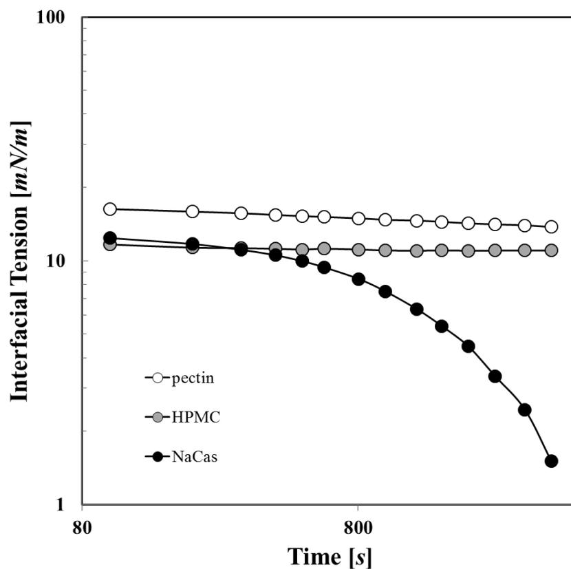
Fig. S2. Behaviour of 2% pectin, HPMC and NaCas (in solution) at the sunflower/water interface.
