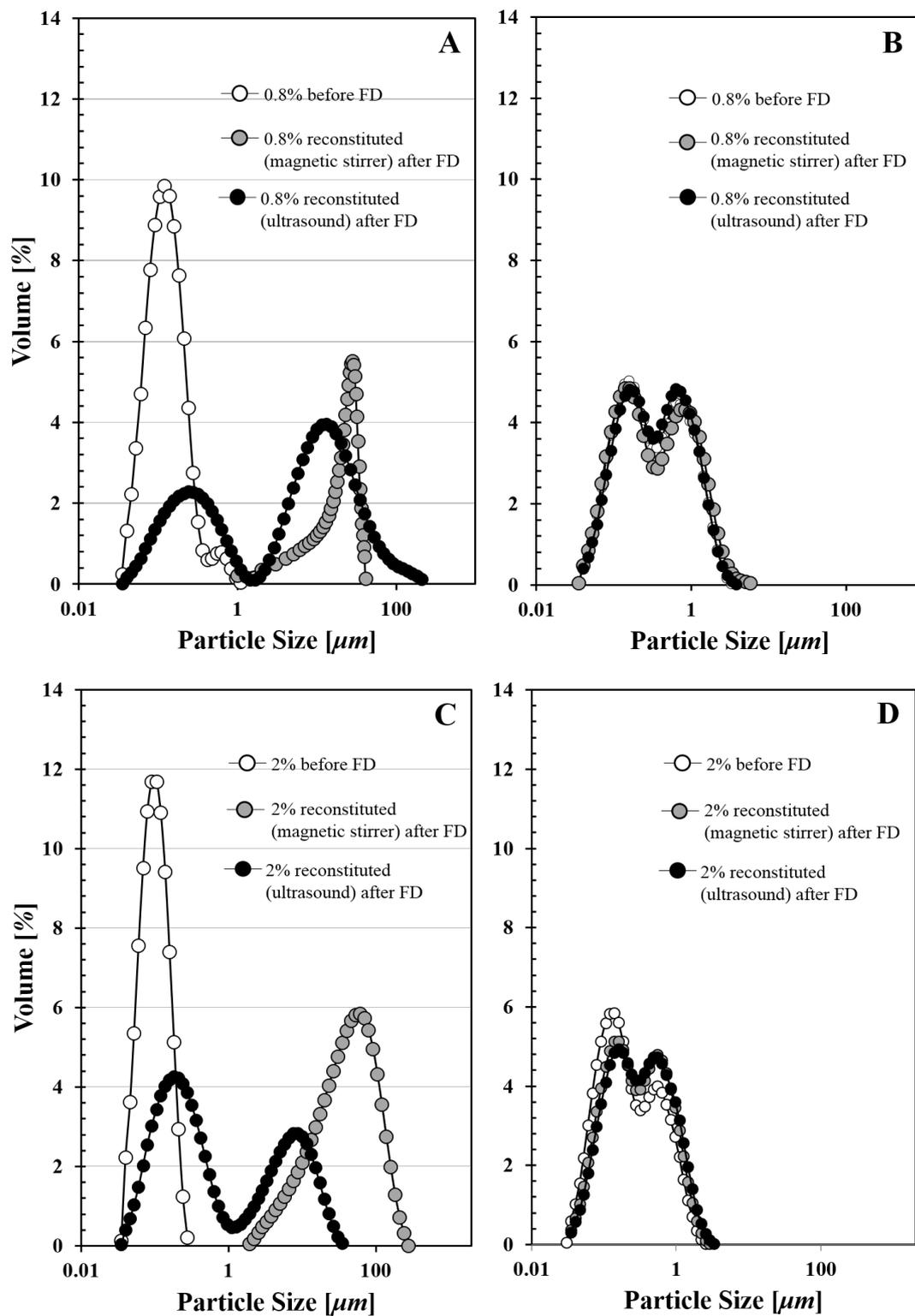
**Fig. 1.** Particle size distributions of solid cetyl palmitate (wax) particles in the presence of 0.8 and 2 %wt Tween 80 (A, C) or sodium caseinate (B, D), before and after freeze-drying (FD) and for two different reconstitution methods.
