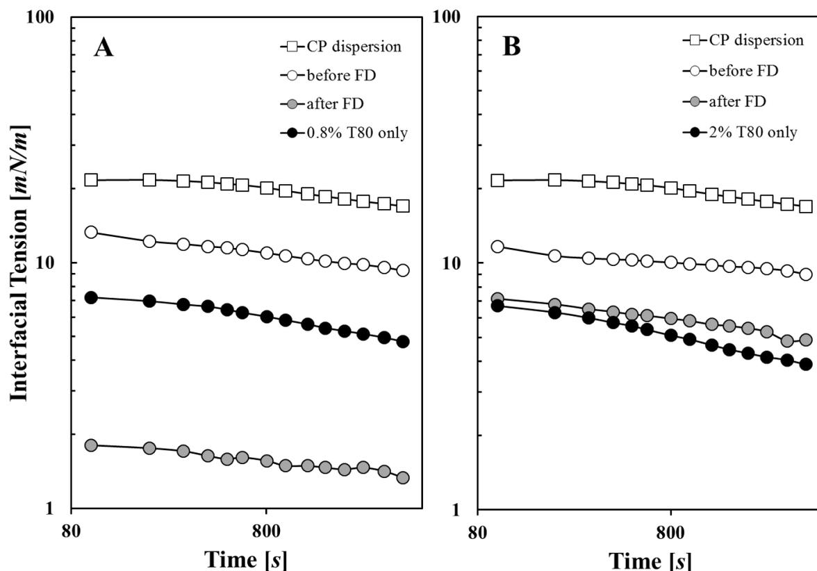
**Fig. 9.** Interfacial tension between sunflower oil and aqueous dispersions of solid cetyl palmitate particles formed in the presence of 0.8 (A) and 2 %wt (B) Tween 80 before and after freeze-drying (FD).
