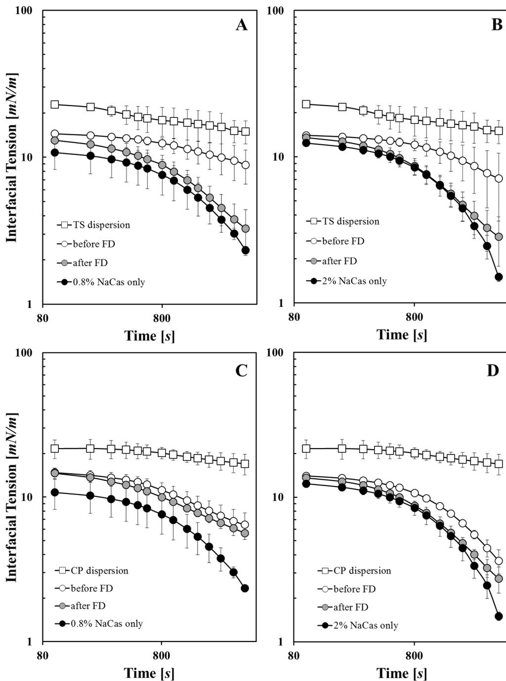
**Fig. 8.** Interfacial tension between sunflower oil and aqueous dispersions of solid tristearin (A,B) and cetyl palmitate particles (C,D) formed in the presence of 0.8 and 2 %wt NaCas before and after freeze-drying (FD). Surfactants in solution are presented on the graph as a reference. All formulations contain 2.5 %wt of lipid material.
