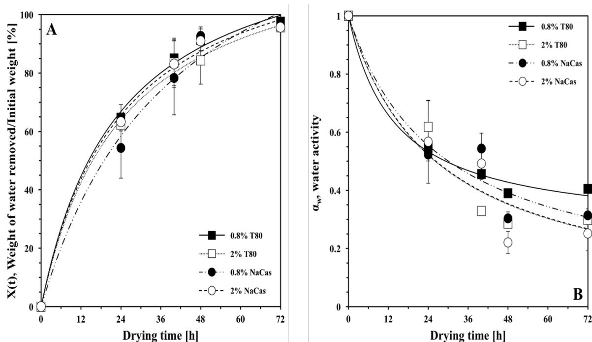
**Fig. 5. A.** Drying curves for different amounts of Tween 80 and NaCas for dried and resuspended cetyl palmitate particles formed in the presence of either surface active species. **B.** Water activity measurements of the dried powders. Measurements were carried out in duplicates with the mean values shown and the error bars representing  $\pm 0.5$  standard deviations.
