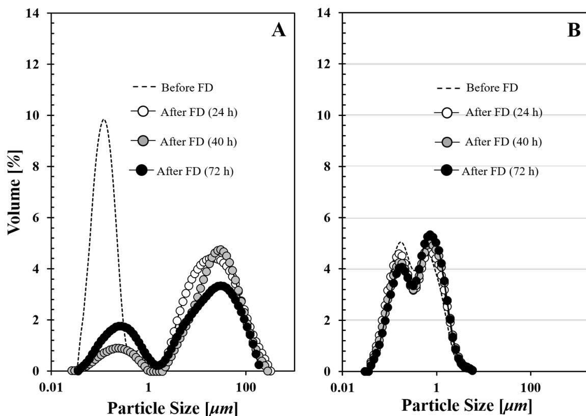
**Fig. 6.** Particle size distributions of dried and redispersed 2.5 %wt solid cetyl palmitate particles produced in the presence of 0.8% Tween 80 (**A**) and 0.8% NaCas (**B**) for different drying times. Original wax particles with the same amounts of surfactants serve as a reference.
