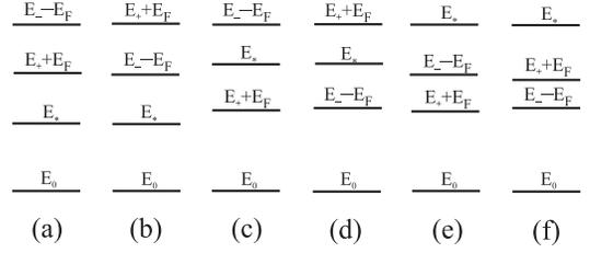
FIG. 6: Feasible energy levels of the molecular junctions in the absence of an applied voltage.  $E_0$ ,  $E_*$ ,  $E_+$  and  $E_-$  are the molecular energies and  $E_F$  denotes the electrode Fermi energy.
