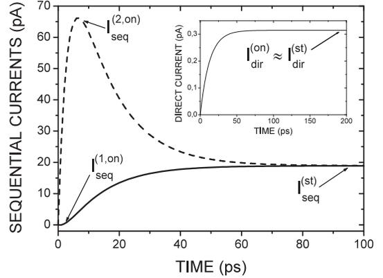
FIG. 8: Off-resonant regime of current formation at a small transmission gap  $\Delta E_{+*}$ .
