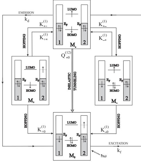
FIG. 5: Transfer routes of the light-induced interelectrode  $\mathbf{12} \rightarrow \mathbf{1^+2^-}$  electron transmission including the participation of the charged molecular states  $M_+$  and  $M_-$ . Within the transmission along the sequential route, the charged states are populated while the same states participate in a virtual form only if the transfer proceeds along the tunnel route.
