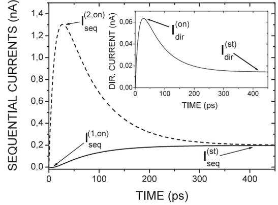
FIG. 10: Single-channel resonant charge transmission with the participation of the charged molecular state  $M_+$  (the energy gap  $\Delta E_{+*}$  is negative). The total current is mainly determined by the sequential components.
