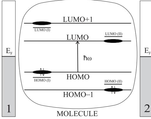
FIG. 1: Possible position of the frontier MOs in the molecule with two terminal sites I and II. Intersite coupling transforms the site MOs into extended HOMO, HOMO-1 and LUMO, LUMO+1. Spots indicate the main location of electron density within the extended MOs.
