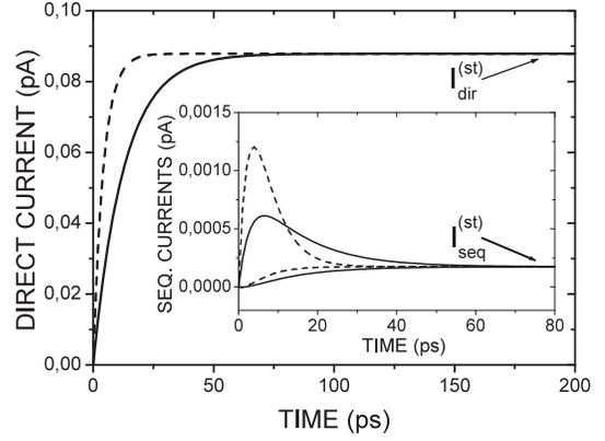
FIG. 7: Transient current components for an off-resonant charge transmission process and at a different intensities of optical excitation. Solid lines:  $k_f = 10^{10} \text{ s}^{-1}$ , dashed lines:  $k_f = 3 \cdot 10^{10} \text{ s}^{-1}$ . Inset: sequential current components  $I_{seq}^{(1)}(t)$  (upper curves) and  $I_{seq}^{(2)}(t)$  (lower curves) approach the common steady state value.
