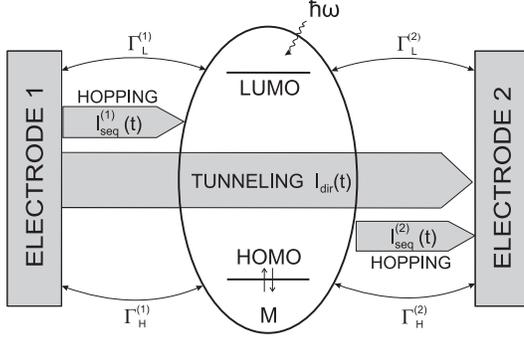
FIG. 2: HOMO-LUMO scheme related to the electron transfer through the **1-M-2** molecular junction. The width parameters  $\Gamma_j^{(r)}$  characterize the efficiency of contact electron jumps as well as of the direct (tunneling) electron transfer. The sequential current components  $I_{seq}^{(1)}(t)$  and  $I_{seq}^{(2)}(t)$  can differ from each other if the junction is transient regime.
