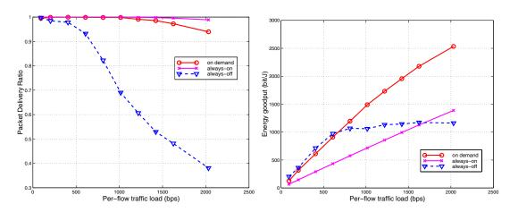
Fig. 6. packet delivery ratio and energy goodput vs. traffic load. 30 on-off connections, on = 10s, off = 100s, 50 nodes, 1500x300 static network
