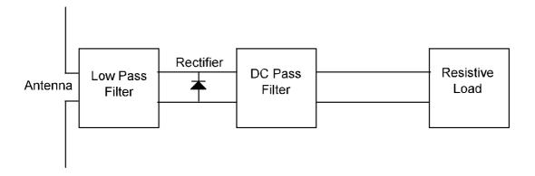
Fig. 1. Block diagram of rectenna and load.
