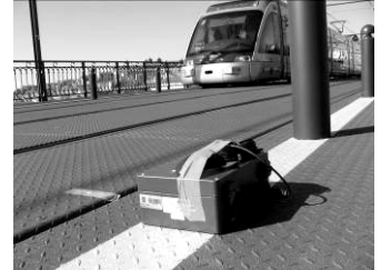
Figure 1 – Ambient Vibration test of a bridge in Porto
