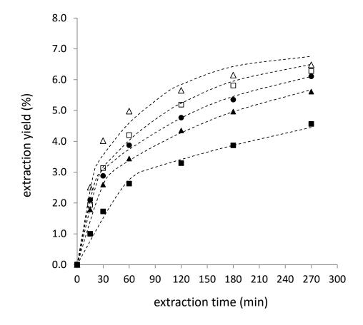
Figure 3. Total extractable material ( $X_o$ ) and marigold solubility ( $Y^*$ ) in supercritical CO<sub>2</sub> at 313 K and 14 MPa. Data represent the OECs obtained at 313 K and 14 MPa in  $V_A$  (2.7x10<sup>-4</sup> m<sup>3</sup>) with different CO<sub>2</sub> flow rates Q = ( $\blacksquare$ ) 2.5×10<sup>-4</sup> kg·s<sup>-1</sup>, ( $\triangle$ ) 5.0×10<sup>-4</sup> kg·s<sup>-1</sup> and ( $\bullet$ ) 7.5×10<sup>-4</sup> kg·s<sup>-1</sup>.
