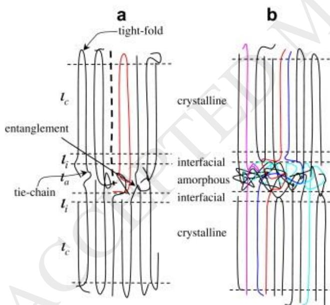
**Figure 11.** Possible mechanism responsible for the brittle-to-ductile transition in: (a) lower molecular mass PPDL and (b) higher molecular mass PPDL. [19], Copyright 2010, Reproduced with permission from Elsevier Ltd.
