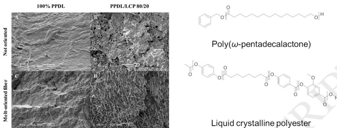
**Figure 12.** Morphology as observed with SEM after blending and extrusion of (A) PPDL, (B) PPDL : LCP 80 : 20 blend, (C) PPDL after melt drawing, and (D) PPDL : LCP 80 : 20 after melt-drawing (draw-ratio of 400). [235], Copyright 2016. Reproduced with permission from the American Chemical Society.
