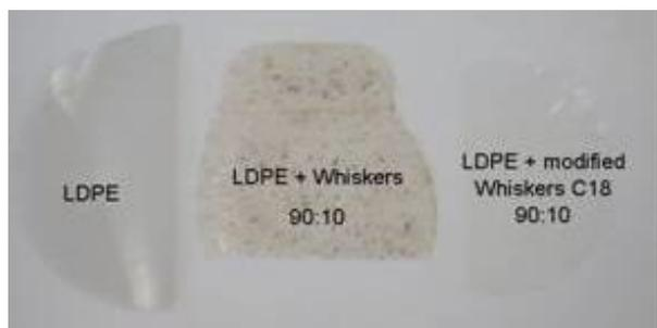
**Figure 10:** Photographs of the neat film and ramie cellulose whiskers based nanocomposite films reinforced with 10 wt% of WRU and WRC18.
