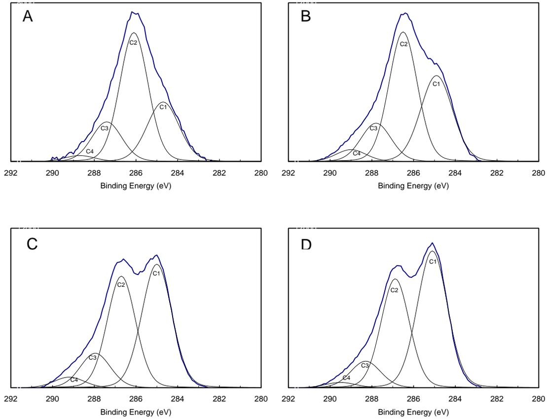
**Figure 4:** Decomposition of C1s signal into its constituent contributions for unmodified ramie cellulose whiskers (A) and modified with hexanoyl chloride (B), lauroyl chloride (C) and stearyl chloride (D).
