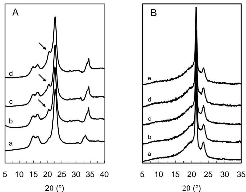
**Figure 6:** Wide-angle X-ray diffraction patterns for ramie cellulose whiskers (A): unmodified (a) and modified with hexanoyl chloride (b), lauroyl chloride (c) and stearyl chloride (d), and nanocomposite films (B): neat LDPE matrix (a) and related nanocomposite films reinforced with 10 wt% ramie cellulose whiskers: unmodified (b) and modified with hexanoyl chloride (c), lauroyl chloride (d) and stearyl chloride (e).
