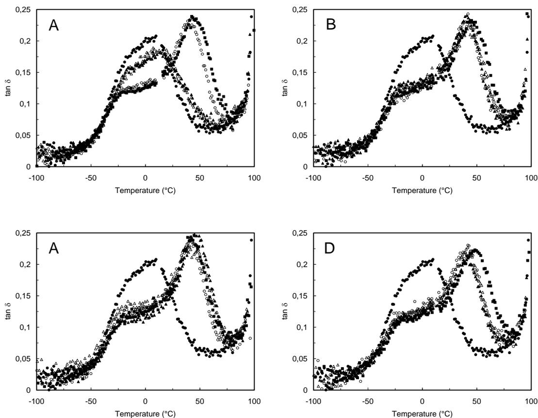
**Figure 13:** Evolution of the tangent of the loss angle ( $\tan \delta$ ) as a function of temperature for the neat LDPE matrix ( $\bullet$ ) and related nanocomposite films reinforced with 3 (A), 5 (B), 10 (C) and 15 wt% ramie cellulose whiskers: unmodified ( $\circ$ ) and modified with hexanoyl chloride ( $\blacktriangle$ ), lauroyl chloride ( $\triangle$ ) and stearoyl chloride ( $\blacksquare$ ).
