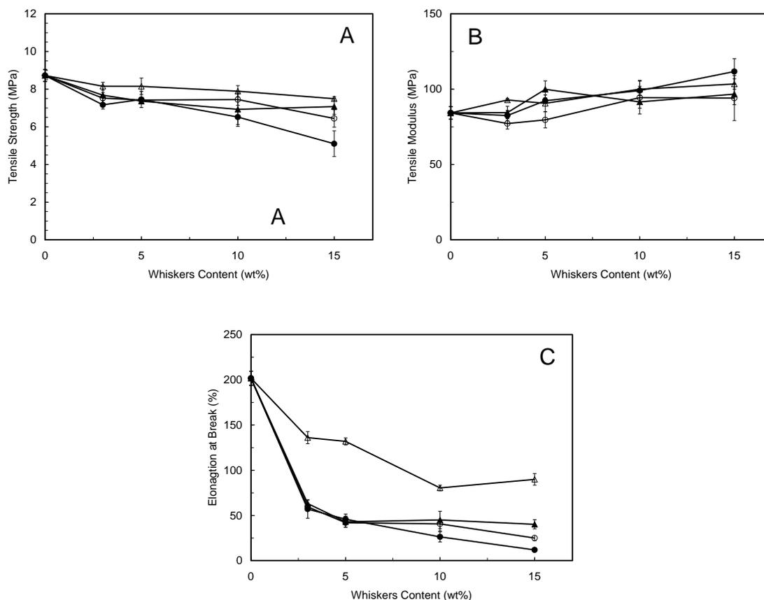
**Figure 14:** Evolution of the tensile strength (A), tensile modulus (B) and elongation at break (C) as a function of the ramie cellulose whiskers content for nanocomposite films reinforced with unmodified (●) and modified with hexanoyl chloride (○), lauroyl chloride (▲) and stearoyl chloride (Δ) whiskers. The lines serve to guide the eyes.
