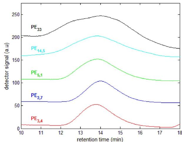
Fig. 1. GPC chromatograms of initial PE samples.
