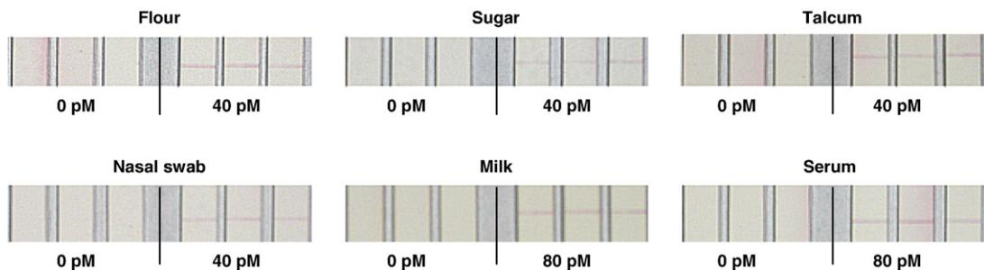
Fig. 3. Limits of detection with the ICT assay in various matrices. The matrices were spiked with the indicated concentrations of BoNT/A complex; the assays were realized in triplicates. Photographs of corresponding capture line signals.
