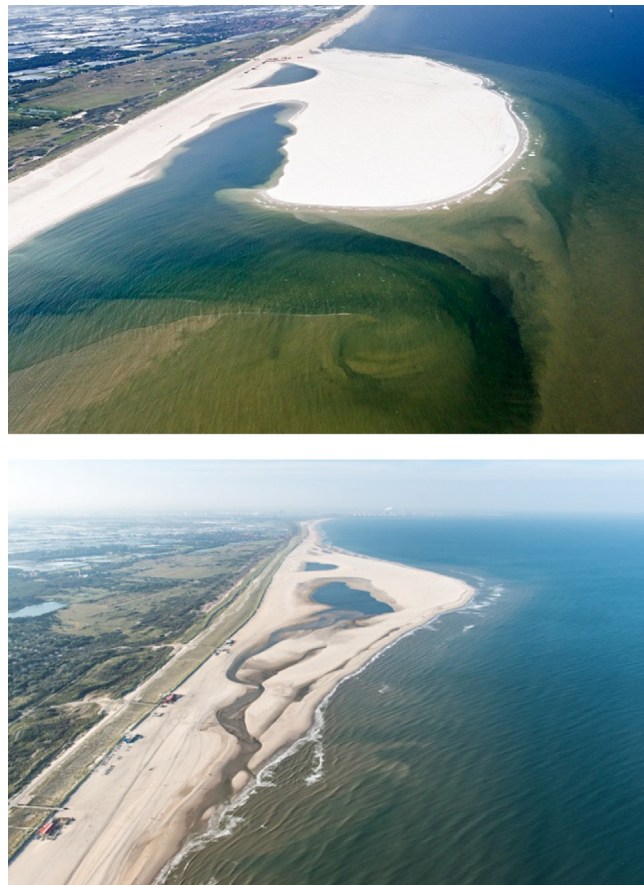
Fig. 8. Upper panel: The Delfland Sand Engine shortly after placement (July 2011). Lower panel: The Sand Engine has evolved into an almost symmetrical salient (October 2013). source: https://beeldbank.rws.nl , Rijkswaterstaat/Joop van Houdt.
