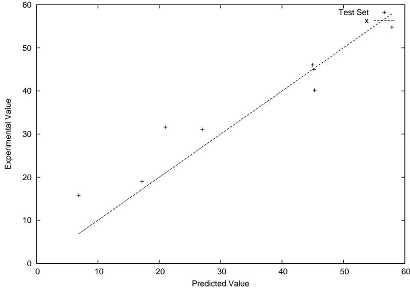
**Fig. 2.** The performance of the back-propagation MLP neural network used to predict the permittivity of the test dataset from the optimised dielectric dataset. This plot illustrates the performance of the first dataset in the cross-validation analysis (See Table 3). An ideal straight line is shown as in the previous figure. The RRS error between experimental and predicted data is 0.63 (dimensionless).
