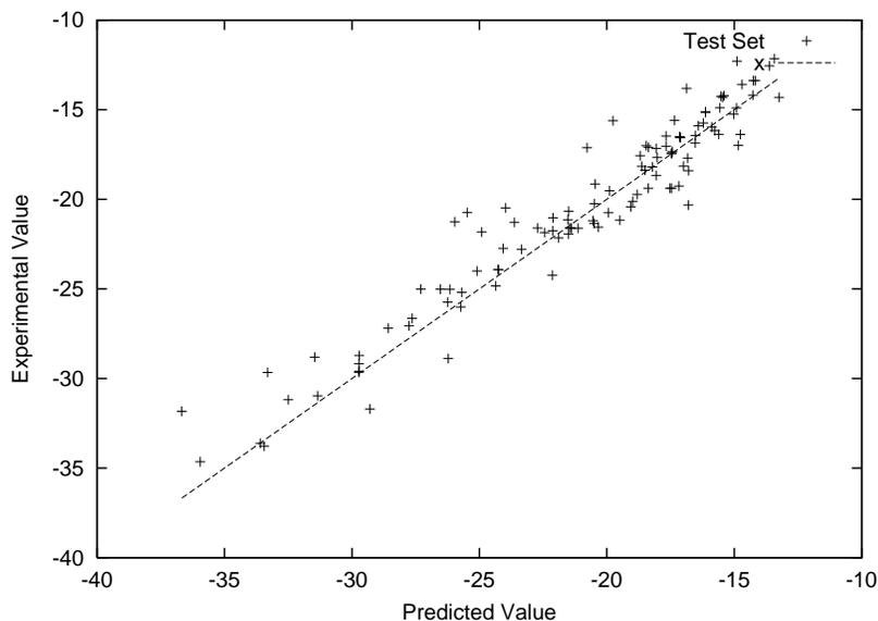
**Fig. 3.** The performance of the back-propagation MLP neural network used to predict the diffusion coefficient ( $\text{cm}^2\text{s}^{-1}$ ) of the test dataset from the ion-diffusion dataset. The RMS error between experimental and predicted data is 0.34 (dimensionless, since the network is trained using the logarithm of the diffusion data).
