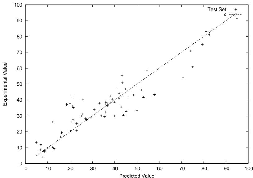
**Fig. 1. The performance of the back-propagation MLP neural network used to predict the permittivity of the test dataset from the full dielectric dataset. This plot illustrates the performance of the second dataset combination in the cross-validation analysis (See Table 1). An ideal straight line with intercept 0 and slope 1 is also shown. The RRS error of the predictions is 0.61.**
