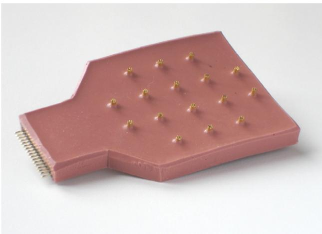
Fig. 1. Two-dimensional 16-channel electrode array used for EMG recordings. The inter-electrode distance is 10 mm. The array was placed parallel to the line from C7 to the acromion.
