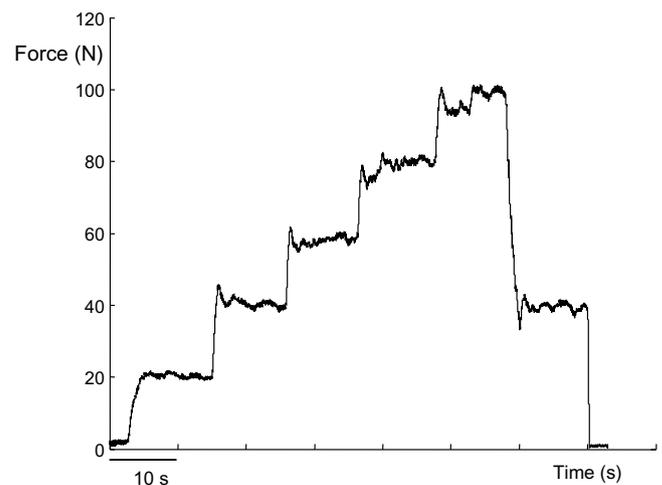
Fig. 3. Typical example of force curve. Force steps of 20, 40, 60, 80 and 100 N were maintained for 10 s each, with 1 s in between for transition to the next step. The sixth step was a repetition of the second step (40 N).
