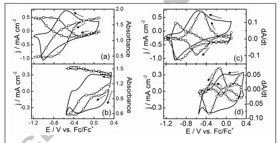
**Figure 8:** Cyclic voltammogram (full line) Absorbance (a and b) and dA/dt (c and d) vs applied potential at 480 nm (open square) and at 660 nm (open circle) for PPy in EMITf<sub>2</sub>N (a and c) and HEITf<sub>2</sub>N (b and d). Scan rate: 50 m V s<sup>-1</sup>.
