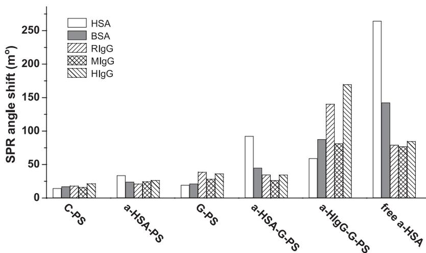
Fig. 5. SPR angle shift as a result of the interaction of different polymersome preparations (C-PS, a-HSA-PS, G-PS, a-HSA-G-PS, a-HIgG-G-PS) and free a-HSA with different immobilized protein spots (HSA, BSA, rabbit IgG, mouse IgG and Human IgG).
