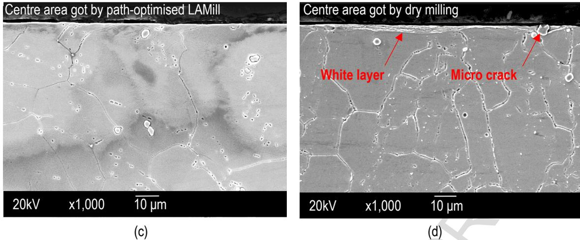
Fig. 18 Microstructure of path-optimised LAMill and dry milling subsurface: at edge area gotten by path-optimised LAMill (a) and dry milling (b), at center area gotten by path-optimised LAMill (c) and dry milling (d)
