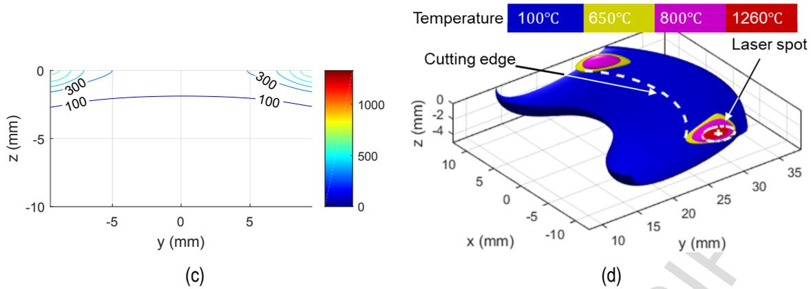
Fig. 4 Predicted temperature distribution for the initially chosen laser trajectory: on the top surface (a), on the depth of cut plane (b), along the cutting cross section(c) and the 3D view (d). Parameters used were: cutting width=19mm, cutting depth=0.26mm, feed rate=948mm/min (0.5mm/tooth) and laser beam diameter=3mm.
