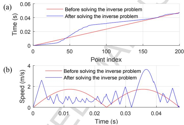
Fig. 3 Comparison of laser scanning trajectories before and after solving the inverse problem by speed optimization: time series  $t_j$  in laser scanning configuration  $(P, x_{bj}, y_{bj}, t_j)$  (a) and laser scanning speed in one scanning cycle (b)
