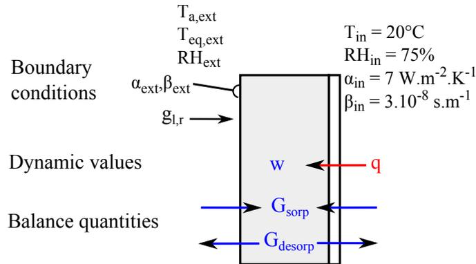
Figure 10: Simulation setup definition of the output notations
