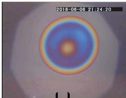
Figure 10. Hexadecane film, stabilized with 1 wt % Span 80, and formed between two aqueous phases, containing 500 mM NaCl. The picture is taken 1 h after the film formation and the colored reflected light indicates film thickness which is \geq 300 nm.
