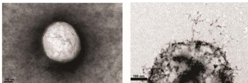
**Figure 4:** Transmission electron microscopy analysis of the optimal formulation of copaiba oil-loaded chitosan- poly (isobutylcyanoacrylate) nanocapsules stained with phosphotungstic acid (2%) at 60 kV (Imagif). Scale bar of 100nm.
