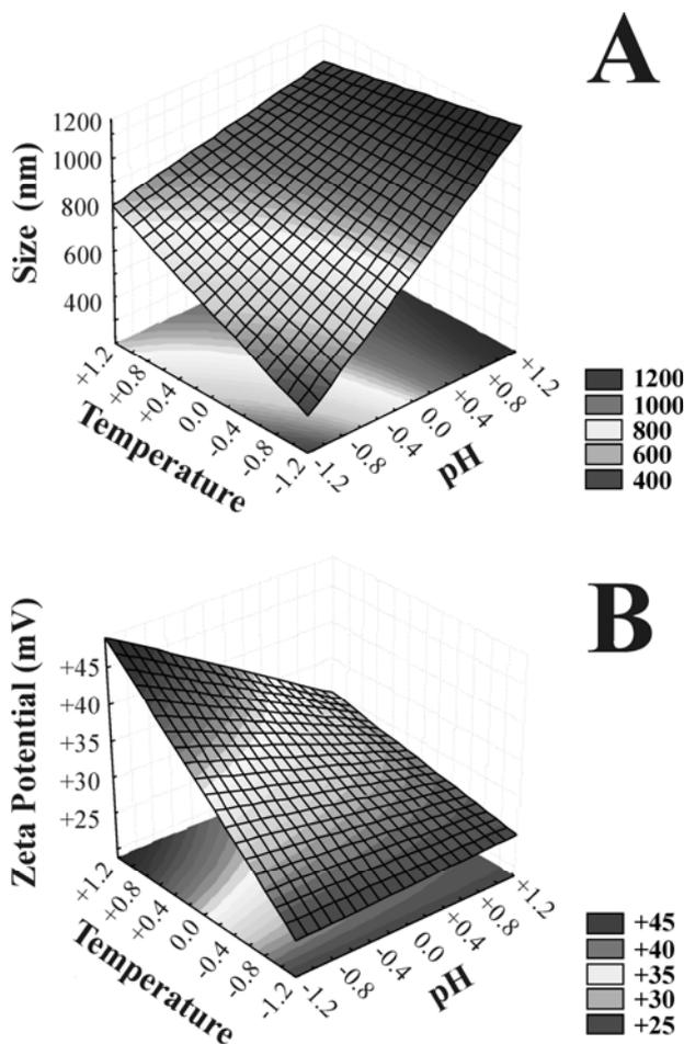
**Figure 3:** 3D Response surface for size droplets (A) and zeta potential (B) variable dependency with temperature and pH independent variables to production of nanocapsules.
