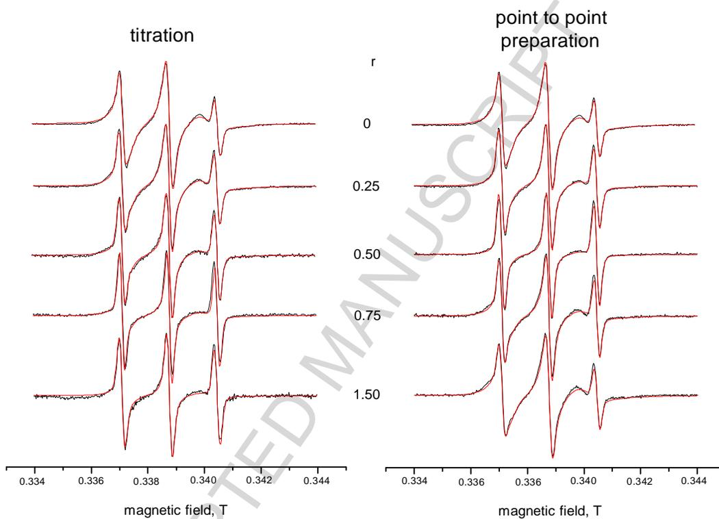
Figure 2. Experimental (black line) and simulated (red line) ESR spectra at 298 K of CAT-12 inserted into dsAT/DOTAP/DOPE lipoplexes prepared by titration (left) and by point-to-point (right) at different  $r$  ratios.
