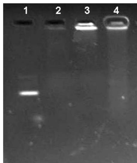
**Fig. 7** Plasma stability of DNA-PLA-PEG-NPs. 1: DNA control; 2: Naked DNA incubated in 10% plasma for 1 h; 3: DNA-PLA-PEG-NPs Control; 4: DNA-PLA-PEG-NPs incubated in 10% plasma for 1 h
