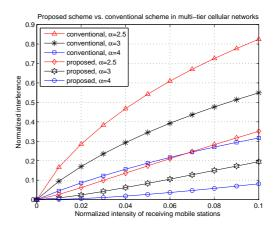
Fig. 2 Interference in a 3-tier cellular network where  $P_k = \{10, 1, 0.1\}, \lambda_k^{\text{BS}} = \{0.01, 0.1, 1\} \text{ and } \lambda^{\text{BS}} / \lambda^{\text{N}}_{-}^{\text{BS}} = 3.$
