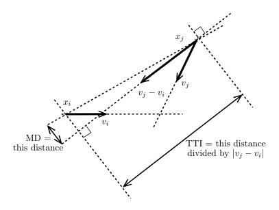
Figure 4: Geometry of a collision: The TTI is the projected distance of the two pedestrians on the direction of the relative velocity  $v_j - v_i$ , divided by the norm of this relative velocity  $|v_j - v_i|$ . The DTI is the TTI times the velocity of the pedestrian. The MD is the projected distance of the two pedestrians on the normal direction to the relative velocity.
