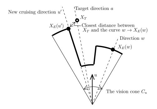
Figure 3: Decision-making phase. The new cruising direction u' is chosen such that the estimated point  $X_E(u')$  in this direction is the closest to the target point  $X_T$ . The tested cruising directions w (with associated points  $X_E(w)$ ) are restricted to the vision cone  $C_u$  of the pedestrian (where u is the current cruising direction).
