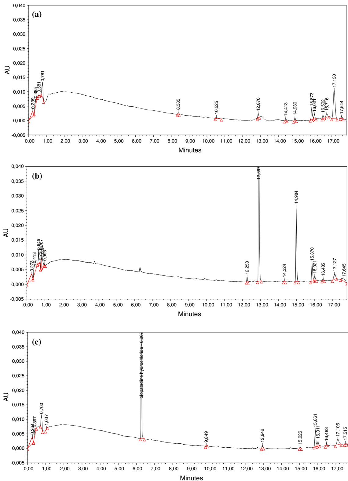
**Fig. 7** Chromatograms of the blank (a), placebo (b) and standard reference solution (c). Blank and placebo solutions show no significant peaks at retention times between 4 and 12 min where the peaks of
