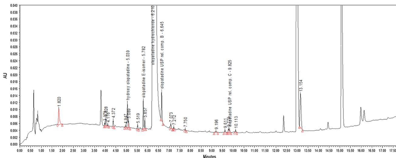
**Fig. 6** Chromatogram of the sample sterilised by heating after 1.5 month of storage at 40 °C/75 % RH. More impurities are present on this chromatogram when compared to the chromatogram of the drug sample sterilised by filtration
