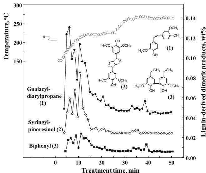
**Fig. 5.** Lignin-derived products (dimeric compounds) from Japanese beech by two-step treatment with hot-compressed water at 10 MPa (230°C for 15 min, 270°C for 15 min) Left axis corresponds to temperature (*open circles*); right axis corresponds to product levels
