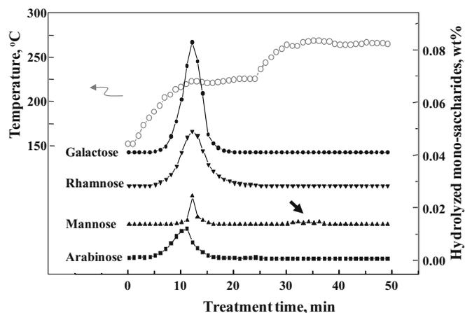
**Fig. 3.** Hydrolyzed monosaccharides produced from Japanese beech by two-step treatment with hot-compressed water at 10 MPa (230°C for 15 min, 270°C for 15 min). Left axis corresponds to temperature (*open circles*); right axis corresponds to product levels. *Bold arrow* indicates presence of mannose
