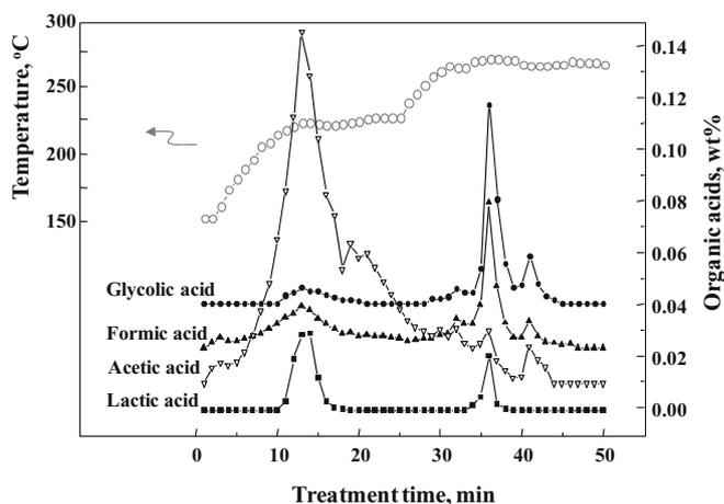
**Fig. 8.** Organic acids produced from Japanese beech by two-step treatment with hot-compressed water at 10 MPa (230°C for 15 min, 270°C for 15 min). Left axis corresponds to temperature (*open circles*); right axis corresponds to product levels
