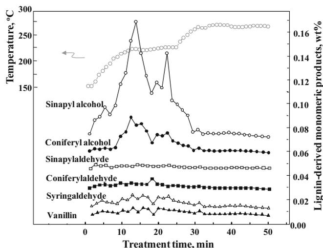
**Fig. 4.** Lignin-derived products (monomeric compounds) from Japanese beech by two-step treatment with hot-compressed water at 10 MPa (230°C for 15 min, 270°C for 15 min). Left axis corresponds to temperature (*open circles*); right axis corresponds to product levels
