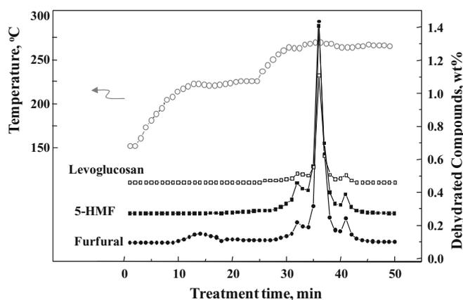
**Fig. 6.** Dehydration products from Japanese beech by two-step treatment with hot-compressed water at 10 MPa (230°C for 15 min, 270°C for 15 min). Left axis corresponds to temperature (*open circles*); right axis corresponds to product levels. 5-HMF, 5-hydroxymethylfurfural
