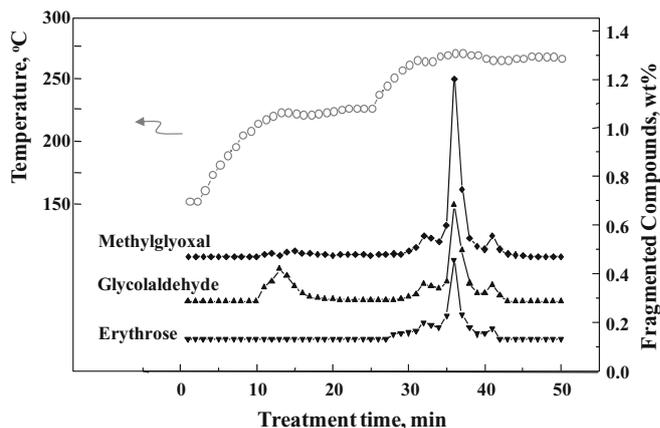
**Fig. 7.** Fragmentation products from Japanese beech by two-step treatment with hot-compressed water at 10 MPa (230°C for 15 min, 270°C for 15 min). Left axis corresponds to temperature (*open circles*); right axis corresponds to product levels
