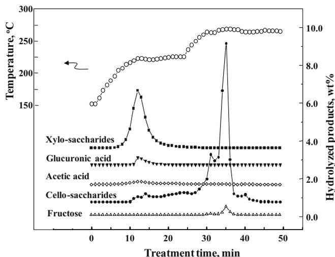
**Fig. 2.** Hydrolyzed products produced from Japanese beech by two-step treatment with hot-compressed water at 10 MPa (230°C for 15 min, 270°C for 15 min). Left axis corresponds to temperature (*open circles*); right axis corresponds to product levels
