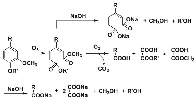
**Fig. 1.** Oxidative degradation of aromatic ring with ozone followed by saponification
