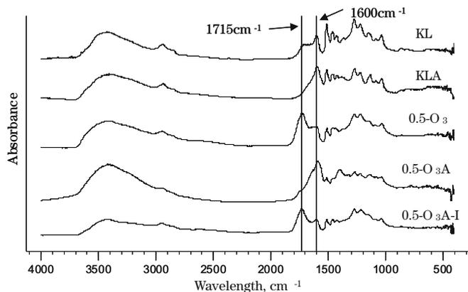
**Fig. 4.** Infrared (IR) spectra of KL, alkaline-treated KL (KLA), lignin treated with ozone for 30 min ( $0.5\text{-O}_3$ ), alkaline-treated  $0.5\text{-O}_3$  ( $0.5\text{-O}_3\text{A}$ ), and alkaline-treated  $0.5\text{-O}_3$  without neutralization after ion-exchange ( $0.5\text{-O}_3\text{A-I}$ )
