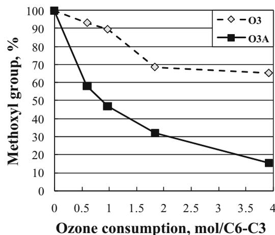
**Fig. 3.** Changes in methoxyl content of ozone-treated KLs before and after saponification. Changes in methoxyl group content were based on the methoxyl content of KL ( $0.63/\text{C6-C3}$ ). Data were calculated based on a molecular weight of 180 for the C6-C3 unit
