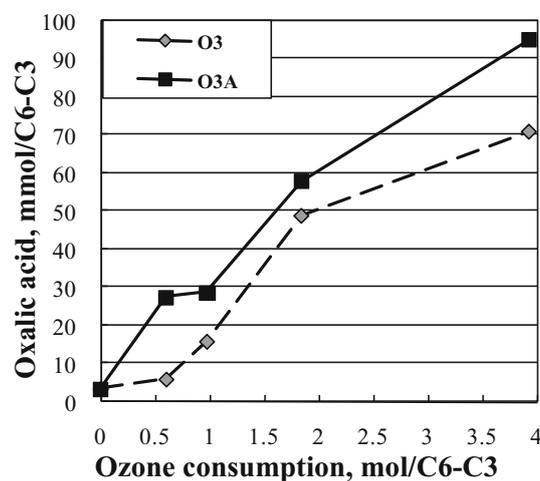
**Fig. 2.** Oxalic acid content of ozone-treated kraft lignins (KLs) before and after saponification.  $O_3$ , Ozone-treated KLs before saponification.<sup>10</sup>  $O_3A$ , Ozone-treated KLs after saponification. A molecular weight of 180 was used for a C6-C3 unit
