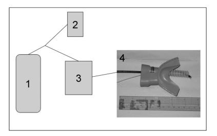
1. Air-puff delivery equipment set-up. 1 = Pressurized air tank; 2 = Digital manometer; 3 = Trigger box with solenoid valve; 4 = Mouthpiece used for routing and placement of the flexible laryngoscope.
