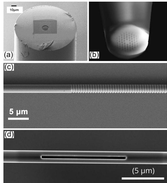
**Fig. 4** A selection of fibre structures milled using the FIB technique: **a** microlens, reprinted from [101], with permission from Elsevier; **b** taper cleaving, reprinted with permission from [102], copyright The Optical Society; **c** fibre Bragg gratings, reprinted with permission from [103], copyright The Optical Society; **d** slotted fibre, reprinted with permission from [48], copyright The Optical Society
