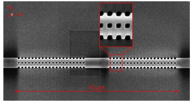
**Fig. 9** SEM image of a 970 nm diameter optical nanofibre milled using a Ga FIB. The structure size measured was  $\sim 141.6 \text{ nm} \times 130.4 \text{ nm}$  with a pitch of  $\sim 326.3 \text{ nm}$
