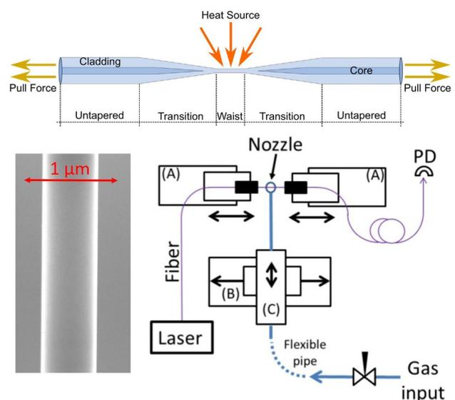
**Fig. 1** Top: schematic of a tapered optical fibre. The optical nanofibre is the ultrathin waist region. Bottom left: SEM image of an optical nanofibre. Bottom right: schematic of a typical fibre pulling rig reprinted from [56], with the permission of AIP Publishing
