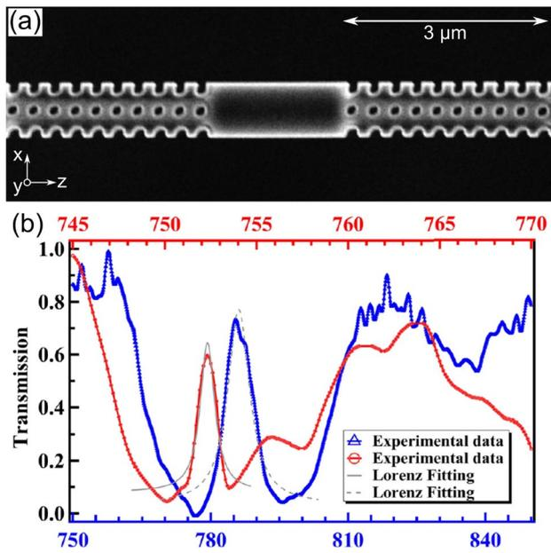
**Fig. 7** Combined structure of a photonic crystal with a Bragg grating. **a** SEM image. The cavity length is 2.2  $\mu\text{m}$ . **b** Transmission spectra per wavelength (nm units) measured for  $x$ -polarisation (red) and  $y$ -polarisation (blue). Reprinted from [51] with the permission of AIP Publishing
