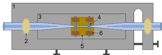
**Fig. 8** Schematic of the base plate with an ITO-coated Si substrate for FIB milling. The numbers in the figure corresponds to the aluminium base plate (1), UV optical glue (2), a removable section (3), a holding fibre (4), the ITO-coated Si substrate (5), and Kapton tape (6)
