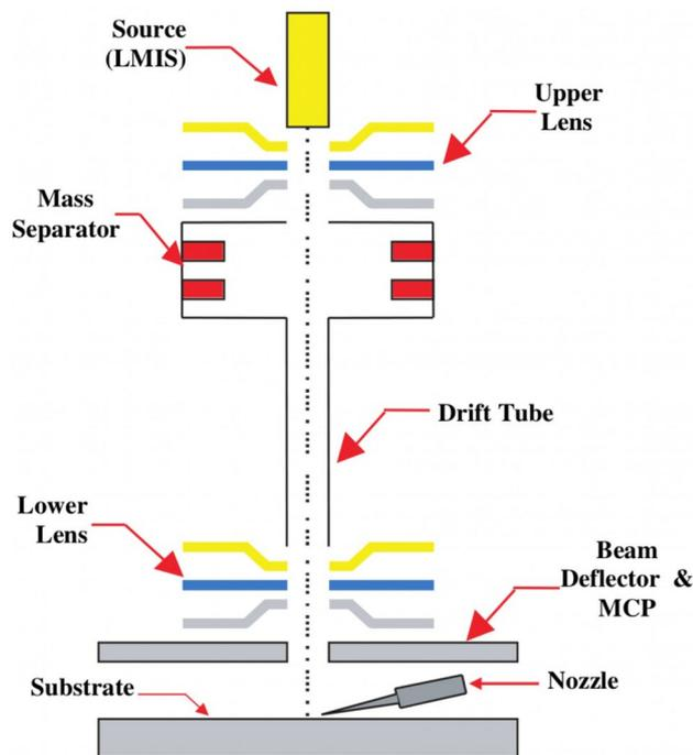
**Fig. 3** Schematic of an FIB system showing the ion source, collimating lens, mass separator, drift tube, focussing lens, beam deflector, multi-channel plate, nozzle, and target substrate. Reproduced with permission from [90], all rights reserved, copyright IOP Publishing
