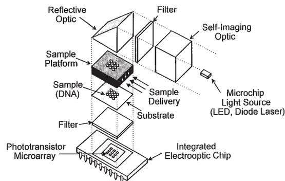
**Fig. 4** Schematic diagram of an integrated DNA biochip system (Source: Ref [173])
