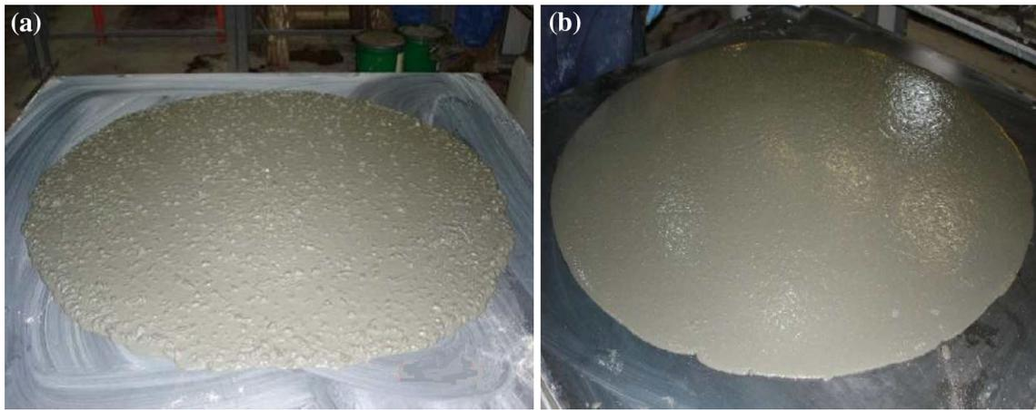
**Fig. 2** Horizontal spread of SCC Mix 2 (a) and Mix 4 (b) with fibres
