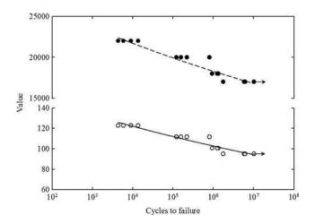
**Fig. 4** Maximum cyclic stress in MPa  $(\bigcirc)$  and maximum load in N  $(\bigcirc)$  as a function of cycles to failure. Arrows indicate indefinite fatigue life
