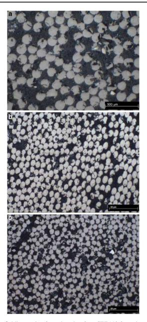
**Fig. 3** Micrographs of samples taken from CF/PA12 femoral stems at various places along the stem's length: (a) proximal region near the neck of the stem with high void content (3–4%); (b) mid-section of the stem with low void content (<2%); (c) distal region of the stem with fairly high void content (2–3%). White spots in micrographs represent carbon fibers. Dark gray patches represent the polymer matrix and black spots indicate pockets of air
