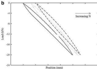
**Fig. 5** Evolution of hysteresis loops for two different tested load conditions: (a) 17 kN (for cycle 30,  $10^5$ ,  $10^6$  and  $5.5 \times 10^6$ ) and (b) 20 kN (for cycle 30, 5000 and  $2 \times 10^5$ )
