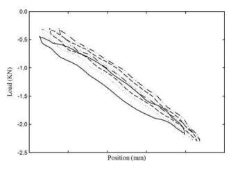
Fig. 10 Evolution of hysteresis loops for a THP stem for cycle 100,  $10^5$ ,  $10^6$  and  $10 \times 10^6$
