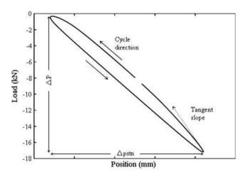
Fig. 2 Schematic drawing of hysteresis loops and measurements. P is considered as load and tangent slope is measured in second unloading part of cycle  $((\Delta \varepsilon/2 = \Delta p/2L))$ , where  $\varepsilon$  is strain, p is position and L is gage length)
