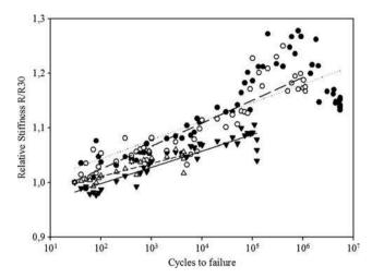
**Fig. 6** Relative stiffness as a function of number of cycles to failure for 17 kN ( $\bullet$ ), 18 kN ( $\bigcirc$ ), 20 kN ( $\blacktriangledown$ ) and 22 kN( $\triangle$ ). Lines show linear regression for each tested condition
