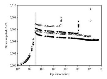
**Fig. 8** Strain amplitude as a function of number of cycles to failure for 17 kN ( $\bullet$ ), 18 kN ( $\bigcirc$ ), 20 kN ( $\blacktriangledown$ ) and 22 kN( $\triangle$ ). Line represents cycle 30 where test was stabilized
