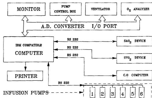
Fig. 1. Hardware and connections of the ACAT system.
