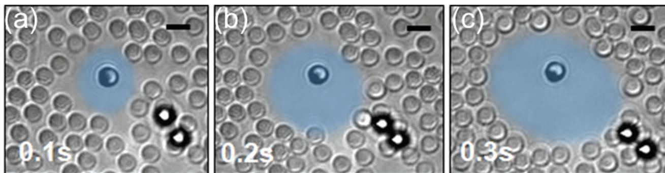
**Figure 5.** The interaction of a single Janus micromotor, fixed to the surface with the passive matrix for the case of high concentrated passive  $\text{SiO}_2$  beads (diameter of 2  $\mu\text{m}$ ). Panels from left to right show the time evolution a) 0.1 s, b) 0.2 s, and c) 0.3 s of the radius  $R$  between the center of the active Janus micromotor and the surrounding passive beads.
