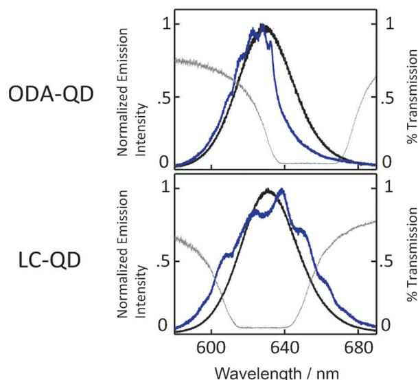
**Figure 6.** Emission spectra for ODA- and LC-QDs dispersed in a cholesteric material (see Experimental Section) at 0.1 wt% and separated into left-handed (black peak) and right-handed (blue peak) components. The cholesteric stop band (transmission spectrum) is also shown (grey) for the right-handed component.
