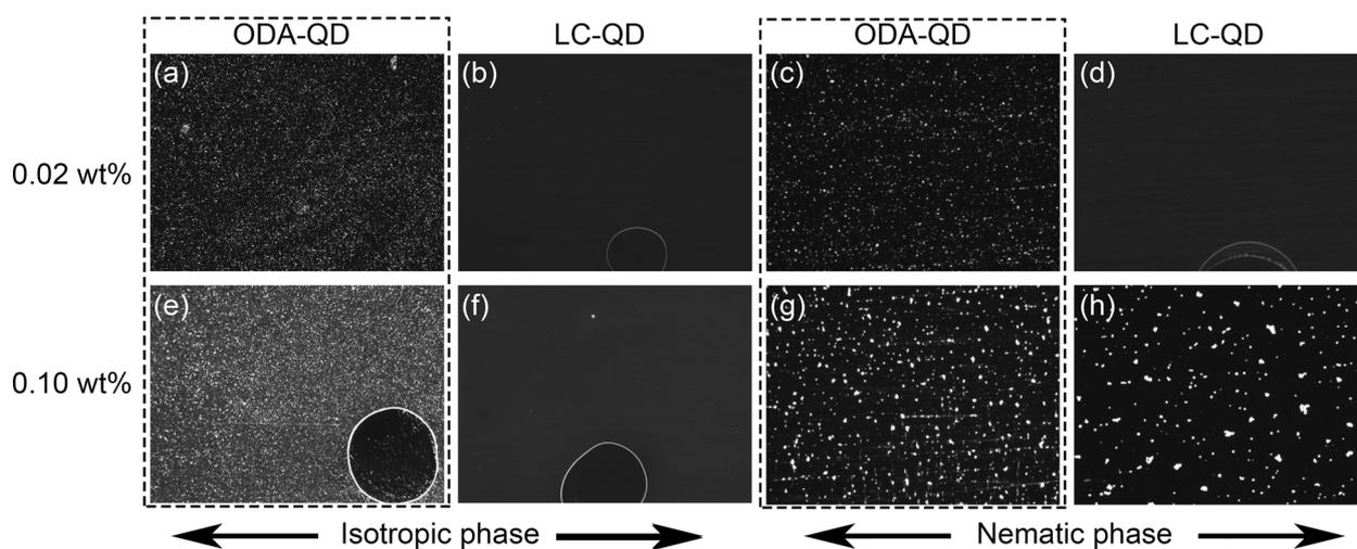
**Figure 3.** Fluorescence microscopy images of different surface-functionalized QDs in the isotropic and nematic LC phase (5CB). a) ODA-QD, 0.02 wt%, isotropic. b) LC-QD, 0.02 wt% isotropic. c) ODA-QD, 0.02 wt%, nematic. d) LC-QD, 0.02 wt%, nematic. e) ODA-QD, 0.10 wt%, isotropic. f) LC-QD, 0.10 wt% isotropic. g) ODA-QD, 0.10 wt%, nematic and h) LC-QD, 0.10 wt%, nematic.
