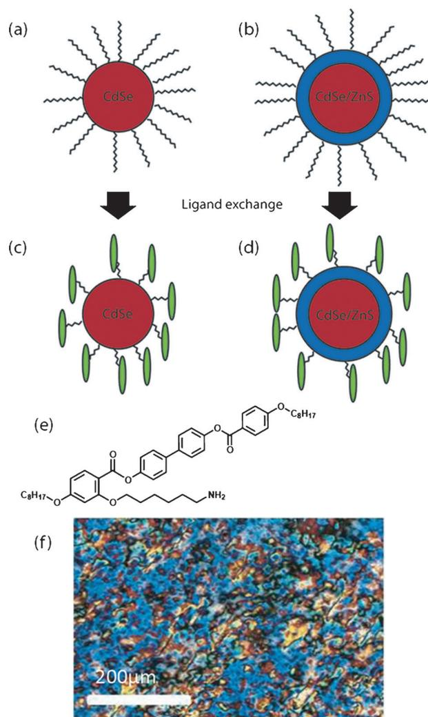
**Figure 1.** Schematic representation of a–d) the different quantum dots used in this study including non-mesogenic ODA ligands and the LC ligand (green). e) Molecular structure of the mesogenic ligand (**11**) and f) nematic phase of **11** at 130 °C, imaged by using polarized optical microscopy.
