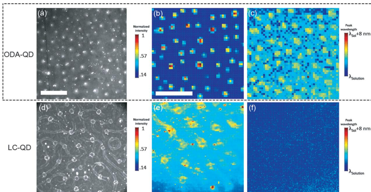
**Figure 5.** Images characterizing large-scale pattern formation in nematic/QD mixtures comparing the ODA and LC ligands. Fluorescence microscopy (a,d), photoluminescence intensity (b,e), and peak emission wavelength (c,f) for ODA-QD and LC-QDs at 0.1 wt% in 5CB are shown (scale bars = 200  $\mu\text{m}$ ).
