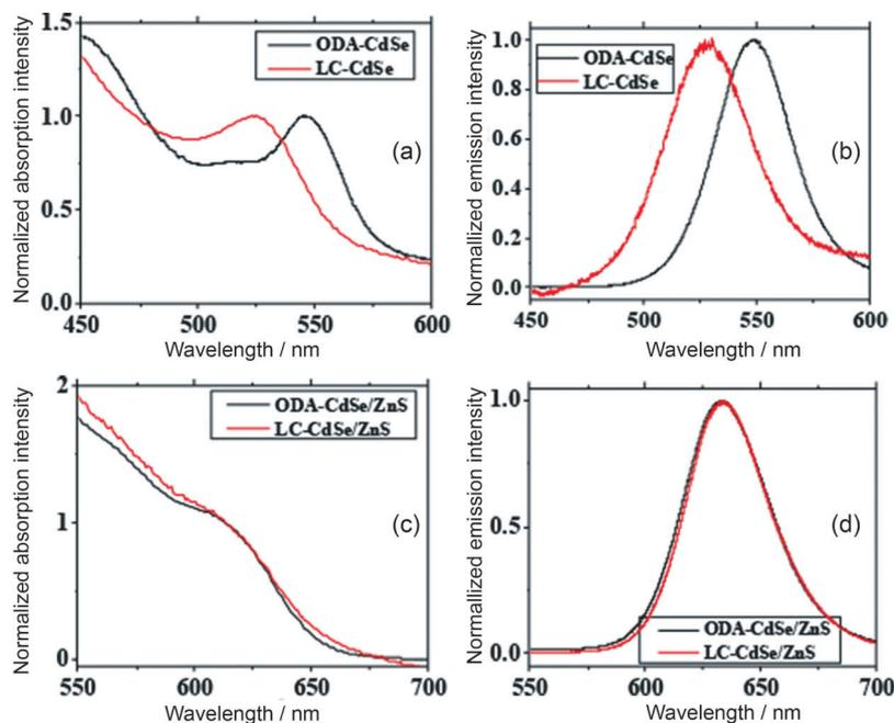
**Figure 2.** Absorption (a, c) and emission (b, d) spectra for ODA- and LC-QDs in toluene with core-only (a and b) and core/shell (c and d) QDs. Each graph shows spectra taken before and after the ligand exchange.
