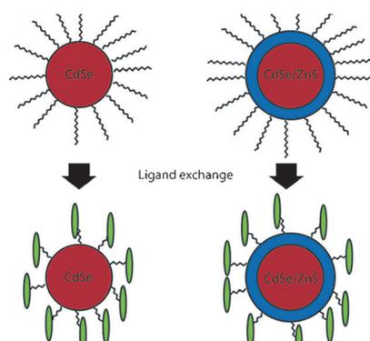
**Dots with liquid-crystalline ligands** are synthesized and dispersed in the nematic and cholesteric phases at different concentrations. Fluorescence microscopy, scanning confocal photoluminescence microscopy, and X-ray diffraction reveal details of the quantum-dot (QD) cluster packing. Spectroscopic measurements demonstrate the applicability of the QDs for photonic applications.
