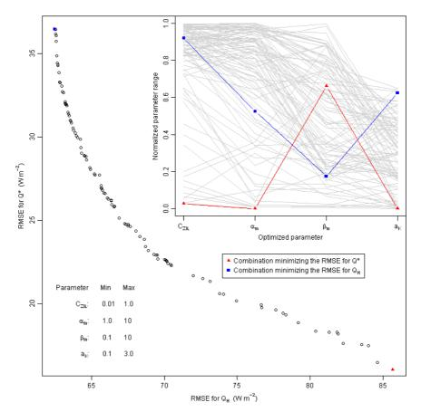
**Figure 9.** Multi-parameter optimization of empirical coefficients  $C_{ZIL}$ ,  $\alpha_m$ ,  $\beta_m$  and  $a_K$ . Inset shows the 100 combinations of parameter values (normalized) selected by MOSCEM. This figure is available in colour online at www.interscience.wiley.com/journal/qj
