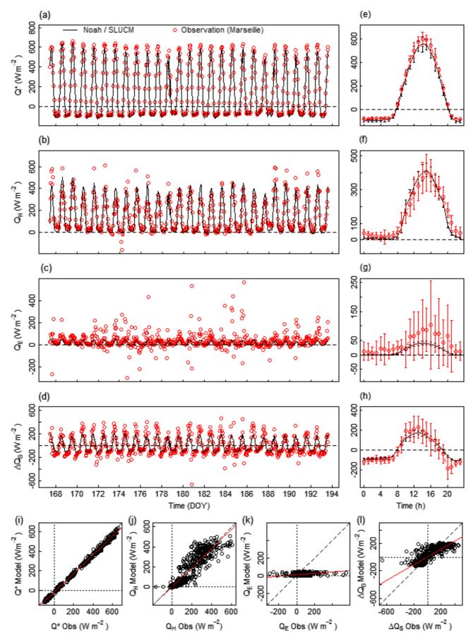
Figure 4. (a) - (d) Time series, (e) - (h) diurnal mean and standard deviation (vertical lines) and (i) - (l) scatter plots of modelled versus observed SEB fluxes for:  $Q^*$  (a, e, i),  $Q_E$  (c, g, k) and  $\Delta Q_S$  (d, h, l). This figure is available in colour online at www.interscience.wiley.com/journal/qj
