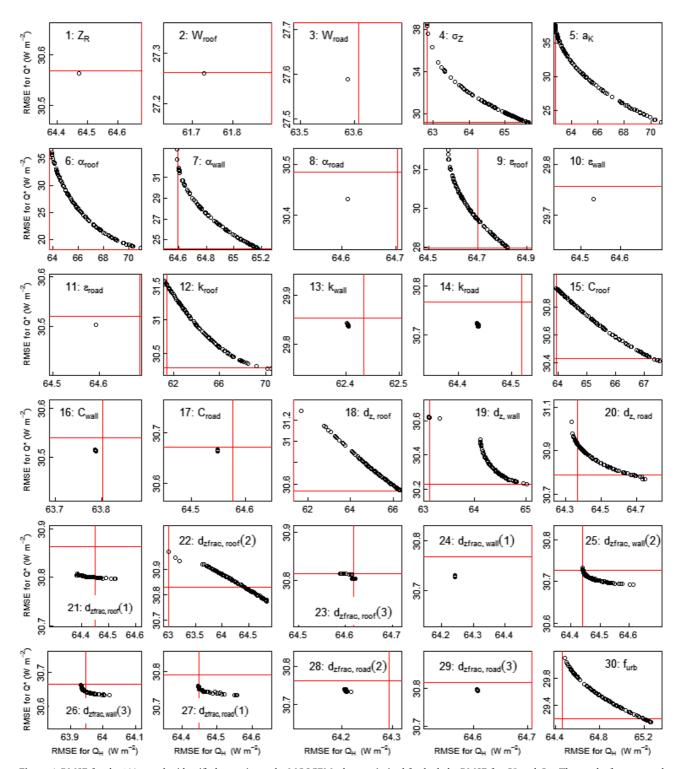
Figure 6. RMSE for the 100 samples identified as optimum by MOSCEM when optimized for *both* the RMSE for  $Q^*$  and  $Q_H$ . The results from control single-objective runs are also plotted (solid lines). Parameters 1 to 29 (SLUCM-related) and the urban fraction ( $f_{urb}$ ) are shown. See Table III for definitions. This figure is available in colour online at www.interscience.wiley.com/journal/qj
