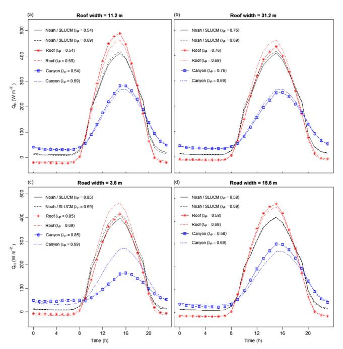
Figure 8. Impact on  $Q_H$  of (a) a 10 m reduction in roof width ( $\lambda_p = 0.54$ ), (b) a 10 m increase in roof width ( $\lambda_p = 0.76$ ), (c) a 5 m reduction in road width ( $\lambda_p = 0.85$ ) and (d) a 5 m increase in road width ( $\lambda_p = 0.58$ ) from the default values ( $\lambda_p = 0.69$ ). This figure is available in colour online at www.interscience.wiley.com/journal/qj
