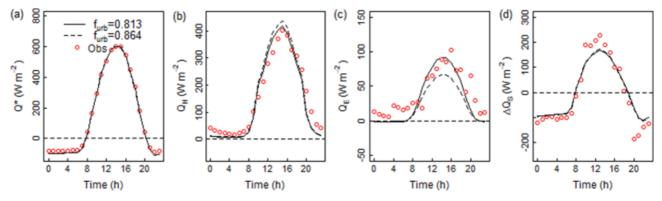
**Figure 10.** Diurnal mean for (a)  $Q^*$ , (b)  $Q_H$ , (c)  $Q_E$  and (d)  $\Delta Q_S$  from two different runs of the Noah/SLUCM ( $\alpha_{roof} = 0.15$ ,  $\alpha_{wall} = 0.15$ ,  $\alpha_{veg} = 0.19$ ,  $R_{cmin} = 40.0$ , LAI=4.0,  $f_v = 0.8$ ) plus  $f_{urb} = 0.864$  (dashed) and  $f_{urb} = 0.813$  (solid). See text for notation. This figure is available in colour online at www.interscience.wiley.com/journal/qj
