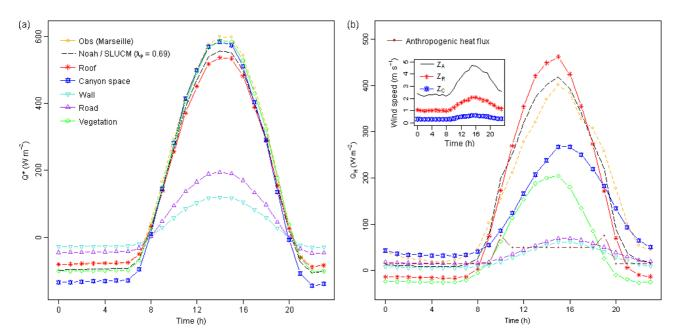
Figure 7. Based on Marseille forcing and observations the contribution of each surface represented in Noah/SLUCM for (a)  $Q^*$ , and (b)  $Q_H$ . Inset to (b): diurnal mean wind speeds at forcing level ( $Z_A$ ), roof level ( $Z_R$ ) and inside canyon ( $Z_C$ ). The anthropogenic heat flux  $Q_F$  (Grimmond *et al.*, 2004) is plotted in (b). This figure is available in colour online at www.interscience.wiley.com/journal/qj
