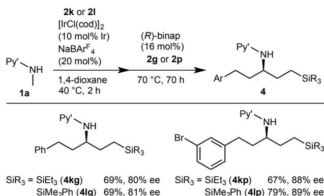
**Scheme 3.** Asymmetric Synthesis of  $\alpha$ -Substituted Amines. *Reaction conditions:* **1a** (0.20 mmol), **2k** or **2l** (0.22 mmol),  $[\text{IrCl}(\text{cod})_2]$  (10 mol% of Ir) and  $\text{NaBAR}^{\text{F}_4}$  (20 mol%) in 1,4-dioxane (0.8 mL) at 40 °C for 2 h. (*R*)-binap (16 mol%) at room temperature for 10 min, and then **2g** or **2p** (0.8 mmol) at 70 °C for 70 h. See the Supporting Information for details.
